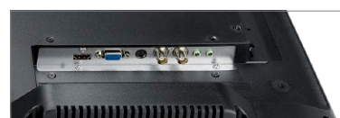
Video versatility, including VGA, HDMI, S-Video and BNC In/Out
