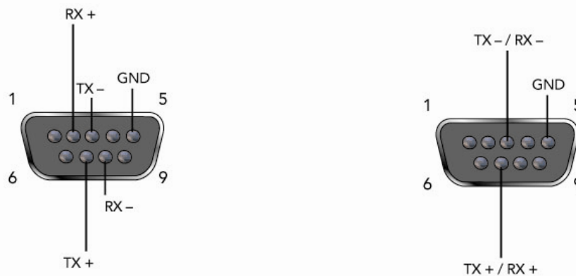
Figure 3-4. RS-422/RS-485 Serial Port Pins
