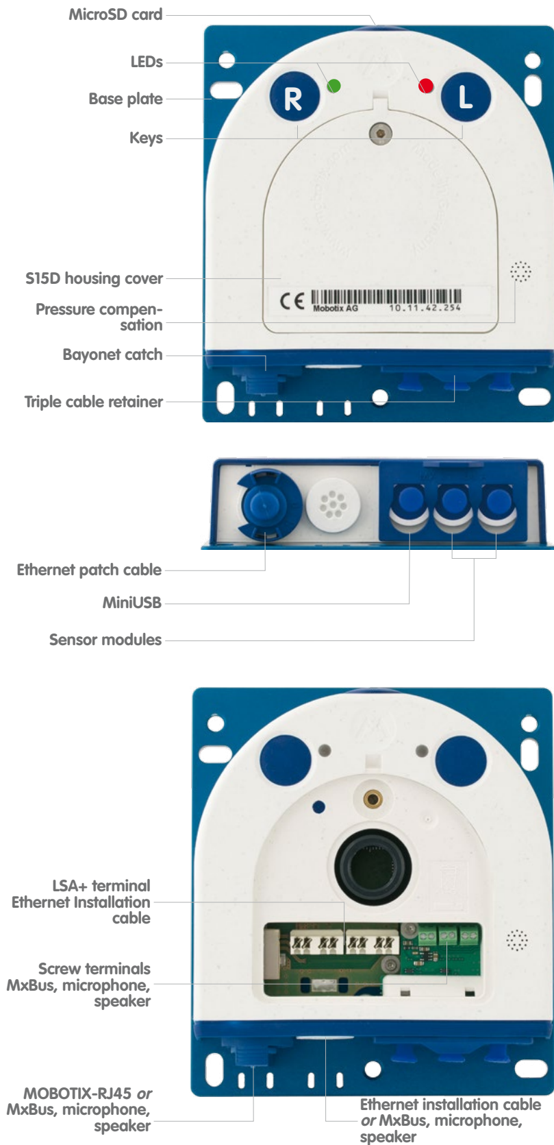
(S15 – Camera housing and connectors, excerpt from the technical documentation)
