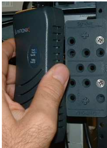
2. Attach the Spider to the bracket's mounting posts
