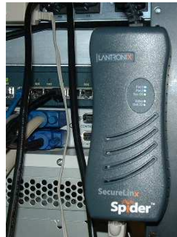
3. Connect cables and the Spider is ready for use!
